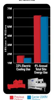
According to a virtual energy audit analysis of Navy Yard Buildings 33 and 36, preliminary estimated energy savings due to the Carrier 23XRV AquaEdge<sup>®</sup> chillers will be in the range of a 33 percent for cooling, and 4 to 7 percent for total facility energy cost.
